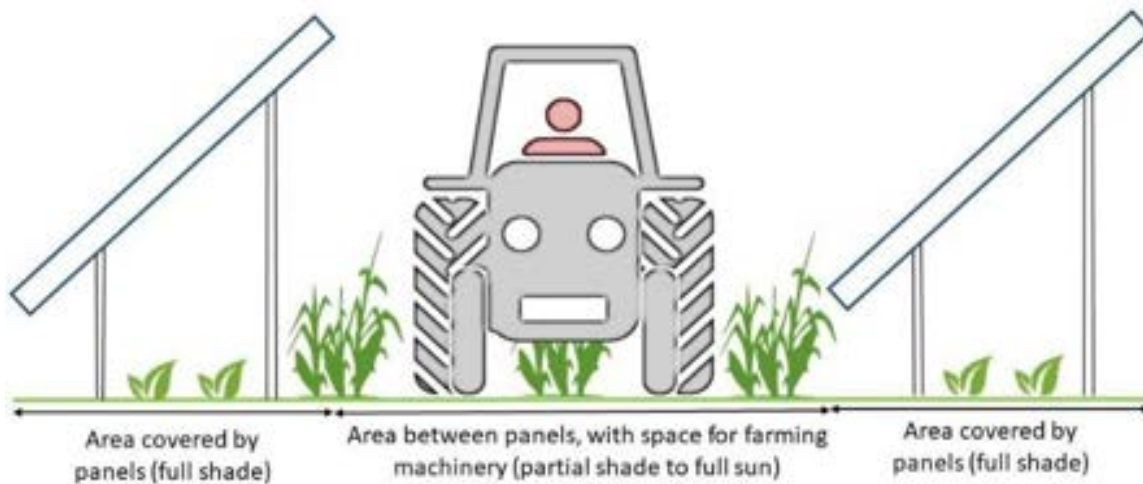
Figure 1: Sample agrivoltaic design. Panel spacing allows farming equipment to pass between rows, with the potential to plant shade-tolerant crops underneath the panels as well as a variety of crops between the rows.
